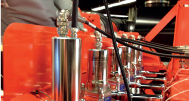
* MOTORTECH flange ignition coil with diagnostic interface
