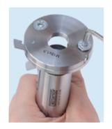
2 Thread adaptors are available in various sizes for the spark plugs that need to be set (M14, M18 or 7/8 in). The adaptors can be mounted or exchanged easily with the included screws and the hex key.
