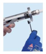
4 Light pressure on the lever is enough to set the electrode gap to the desired distance with the help of a feeler gauge.
