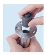
1 The tool is first fitted with the base insert that fits the corresponding spark plug.
