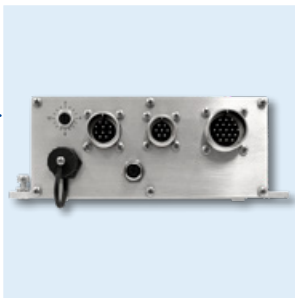
Due to the same connector configuration, the existing input and output wiring can be re-used. Additional connectors for CAN Bus (PowerView3) and analog input (DetCon20) connection.
