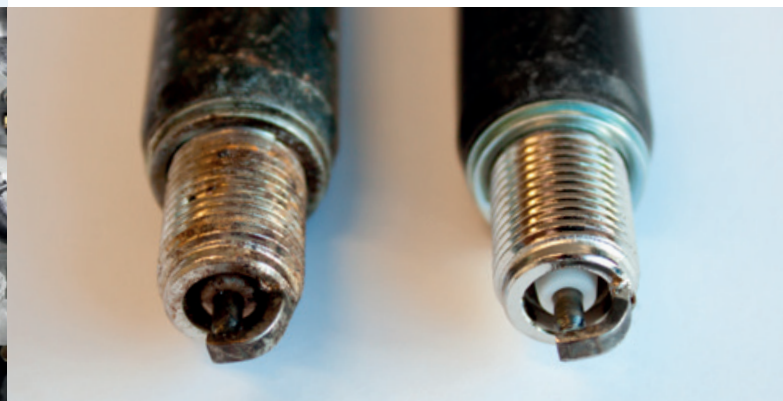
Spark plug after use and after cleaning
