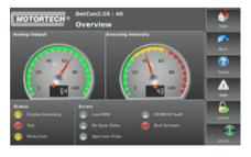
Overview Screen shows the most important operating data of the connected DetCon control unit.
