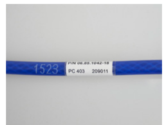
NEW MARKING METHOD WITH WRAP AROUND LABEL APPLIED TO THE IGNITION CABLE
