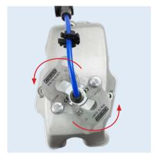
To unlock the spark plug lead the two screws just have to be loosened. The safety flanges can now be turned aside on the flange support.
