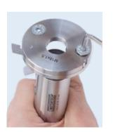
Thread adaptors are available in various sizes for the spark plugs that need to be set (M14, M18, 7/8-18 or M22). The adaptors can be mounted or exchanged easily with the included screws and the hex key.
