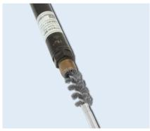
Cleaning of extended barrel spark plug
