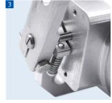
End stop and screw for idle speed adjustment
