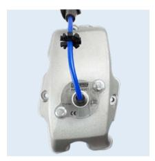
The flanges with the locked spark plug lead are fixed on the valve cover with two screws to prevent the release of components from the spark plug well.
