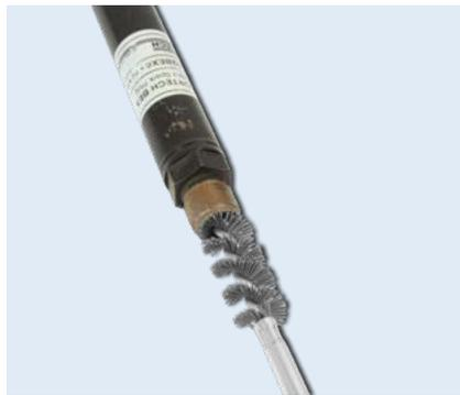
Cleaning of extended barrel spark plug
