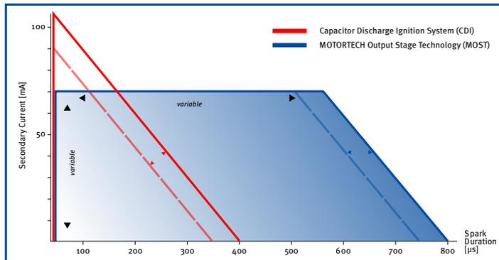
These requirements can only be met by precision ignition behavior and efficient control of the ignition spark. MOTORTECH Output Stage Technology (MOST) was developed by MOTORTECH for this.
