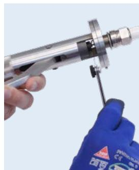
**4** Light pressure on the lever is enough to set the electrode gap to the desired distance with the help of a feeler gauge.
