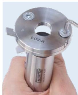
**2** Thread adaptors are available in various sizes for the spark plugs that need to be set (M14, M18, 7/8-18 or M22). The adaptors can be mounted or exchanged easily with the included screws and the hex key.
