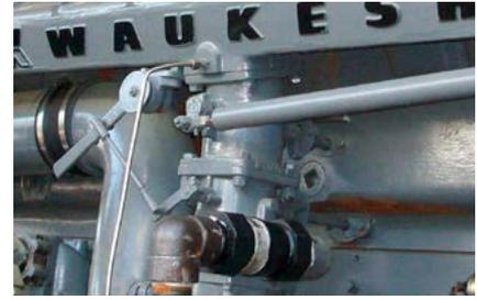
Based on its proven design, MOTORTECH offers a special throttle body series for WAUKESHA® VHP series in-line and V-engines. Designed as a replacement and plug-and-play solution, the throttle bodies perfectly fit the position of the original part below the intake manifold.
