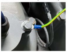
Connect the coaxial cable with the aid of the BNC connector to an oscilloscope or to the SparkView high voltage indicator from MOTORTECH.
