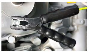
Design with eyelet: For grounding, use the eyelet at the high voltage clamp's grounding cable. Make sure that the eyelet is securely fastened to the grounding point.
