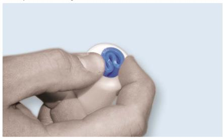
4. Carefully press the silicone seal into the nut using the screw driver.
