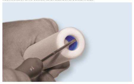
2. Lever off the ring with the screw driver.
