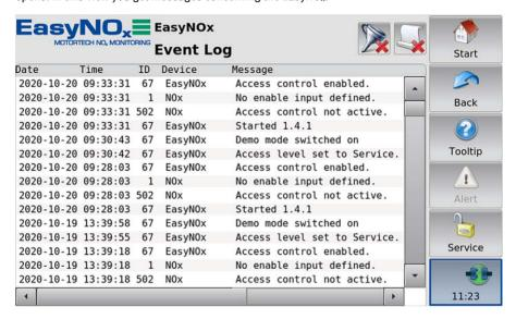
The following data is displayed: date (YYYY-MM-DD) and time (HH:MM:SS) of the entry, node ID or internal sequential number of the device, device name and the accompanying message. A maximum of 1,000 messages are displayed and stored by the EasyNO<sub>x</sub>. Older messages are deleted.
