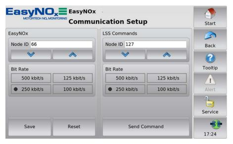
In this view, settings can be made within the CANopen® network to which the EasyNO<sub>x</sub> is connected via the CAN bus interface CAN<sub>1</sub>.
