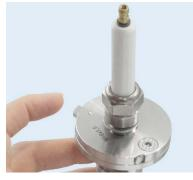
8. Insert the feeler gauge 4 with the corresponding blade for the desired gap between ground electrode and center electrode. Bear in mind that, after pressing, the ground electrode may spring back slightly in certain cases. Rotate the spark plug, if necessary.
