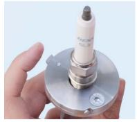
8. Insert the feeler gauge 4 with the corresponding blade for the desired gap between ground electrode and center electrode. If necessary, rotate the spark plug.
