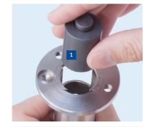
3. Put on the thread adapter that suits your spark plug thread and screw the thread adapter tight with the supplied hexagon socket head cap screws M6x10. Use the supplied hex key SW4 for this.
