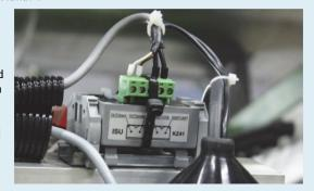
Note that the contacts of the connector are bare and must be protected against moisture and contamination. If the engine should be in such a location, the ignition sensor unit (ISU) can, for example, be mounted in a junction box or housed in a control cabinet.
