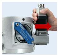
6. While holding the adapter plate in this position, tighten the screws of the adapter plate with a torque of 10 Nm (7.4 lb-ft).
