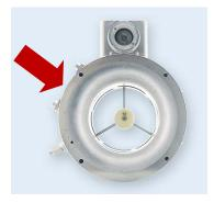
2. Open this gas inlet by removing the cover or the flange.
