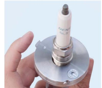
8. Insert the feeler gauge **4** with the corresponding blade for the desired gap between ground electrode and center electrode. If necessary, rotate the spark plug.
