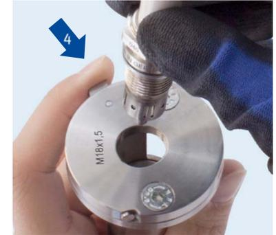
7. Let the lock bar go to fasten the spark plug.
