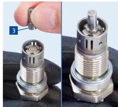
5. To insert the spark plug, press the lock bar <sup>4</sup> to the limit and hold it down.
