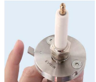
10. Adjust the electrode gap as desired by softly pressing the lever.
